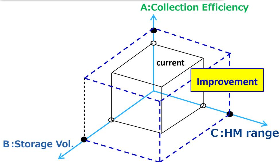
HM range\*; heat medium temperature drop between inlet to and outlet from WFC
