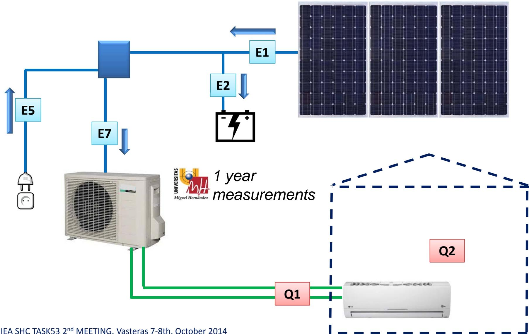
*PV driven solar heating system of a
