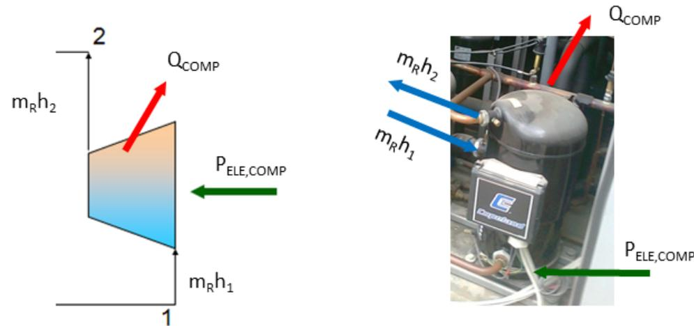
$$P_{\text{ELE,COMP}} = m_R \cdot (h_{20} - h_{11}) + Q_{\text{COMP}}$$
