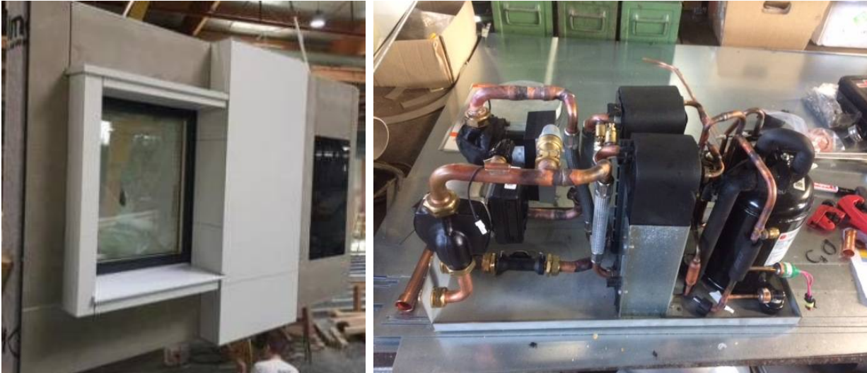
Figure 7 – Experimental model of a façade element with vertical duct where vertical piping and a small-scale heat pump are integrated (left), small-scale heat pump for façade integration (right), picture source: Kulmer Holz-Leimbau GmbH (left) and Vaillant GmbH (right)
